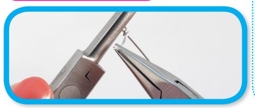
Save time and frustration by investing in a quality pair of cutters such as the Italian Super Flush Cutters. A nice flush cut should be perfectly flat, with no points or jagged edges. This will make your finished jewelry look much nicer and will significantly reduce your filing and finishing time.
