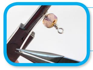
Grip the end of the wire with your Baby Wubbers Chain Nose Pliers, cross it up next to the edge of the jaw of the Wubbers Looping Pliers. Keeping the wire taut as you wrap will allow the wire to glide into place, forming a perfect wrap. There should be enough room to wrap approximately 2 ½ times. If a little more space is needed for the wrap, give the bead a quick tug, and this will allow for additional space to wrap.
