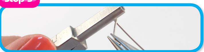
Using a pair of Baby Wubbers Chain Nose Pliers, grip the short end of the wire, cropping as shown. Pull snugly up against the edge of the concave jaw of the Looping Pliers. This will ensure that your loop is properly sized and perfectly round.
