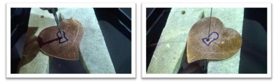
Drill a hole using a small drill bit, insert the saw blade into the hole, and saw out the lock piece.
