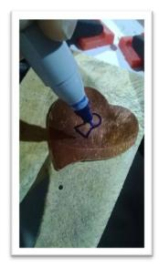
Draw the shape of a lock in center of the heart. (This can be freehanded.) Use a center punch to make a small divot. This so the drill does not skate across the metal and scar it.
