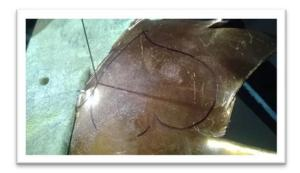
Saw out the shape as close to the line as possible. File, as needed, to help better form the shape of the heart and sand the edges and top smooth.
