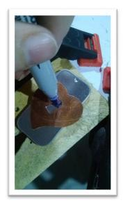
Using the cut out from the heart, trace the lock shape onto the top of the tin so that it lines up with the lock on heart. Pierce and saw out the lock piece from the tin top. (See step 2)
