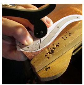
Here are the two sawn pieces. Do not remove the paper just yet! The paper is needed to mark the rivet holes for drilling.
