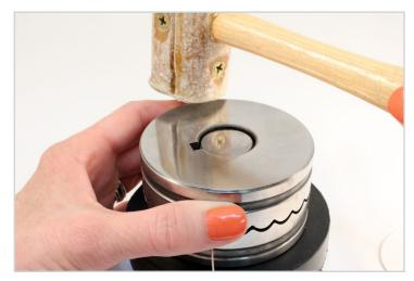
Helpful Tip: Check the progress of the wire as you hammer it in the Wubbers Press. It is easy to create the waves in the 20-gauge wire using moderate pressure with the hammer. If excessive force is used, you may inadvertently flatten the straight end of the wire that will form the post of the earring.
