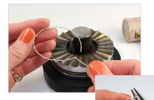
7. Remove the wire from the press. Using the Baby Wubbers Round Nose Pliers, roll a small round loop on one end of the wire.
