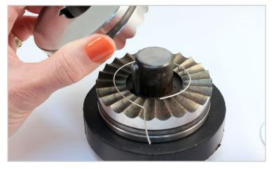
**5.** Working with one wire at a time, center the round part of a wire circle on the bottom half of the Wubbers Bangle Press as shown. The straight end of the wire should lay down in one of the grooves so that it will remain straight.
