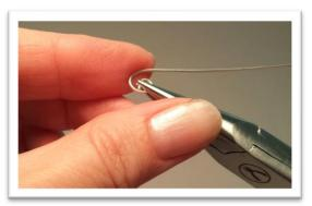
Continue bending the wire into a spiral going around twice. Remove any tool marks if needed by lightly rubbing with fine steel wool.
