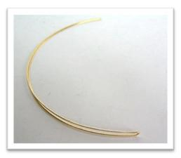
**Step 3.** Grip the U-shaped piece of wire in the center with the Wubbers Classic Medium Flat Nose Pliers as shown. Grasp the wire to the left of the pliers, and gently bend upwards to form a "V."
