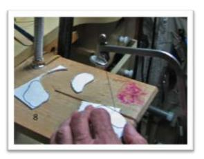
**Step 11.** Remove saw marks or irregularities with the Habilis file. File in a rotary motion, refining the shapes.
