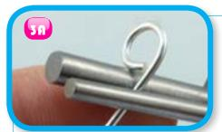
Forming the Second Loop To form the center loop of each link, you will the wire around the small jaw, continuing to
