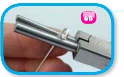
Wubbers Medium Bail Making Pliers (Photo larger jaw (6B). Roll the pliers away from you, the loop in the jaws of the pliers, making sure make a hook (6C).
