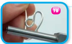
you, grip the wire so that the jaws are even with the edge of the first loop as shown in Photo 7A. Begin to rotate the pliers away
